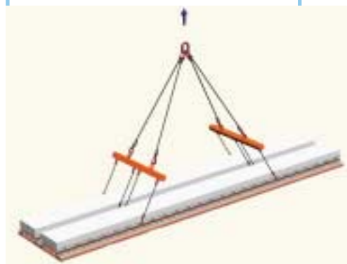
Fig. 10- Sollevamento con bilancino. Handling of the panels with a lifting beam.
